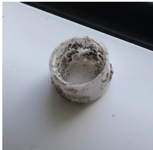
Picture 1 – Crucible after the measurements the residual mass in 950°C above 75% of initial mass.
